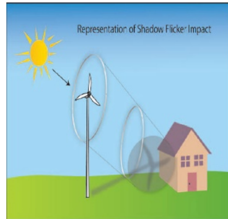
Figure 8: Depiction of how shadow flicker may occur during periods when the sun is behind the WTG
