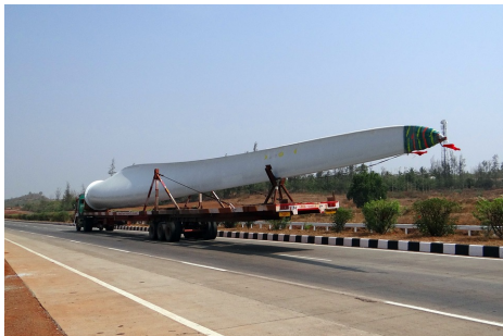
Figure 9: Example of WTG blade being transported to site via abnormal load transporter
